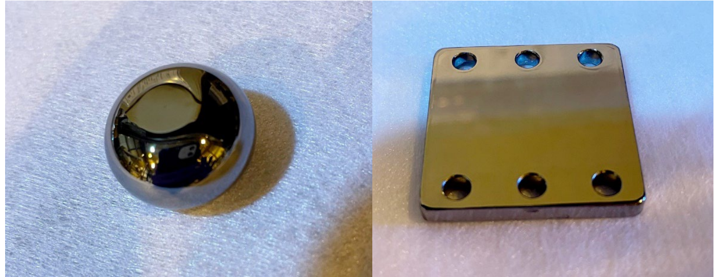
Conductive coating: Cu-Ge coated PMMA
