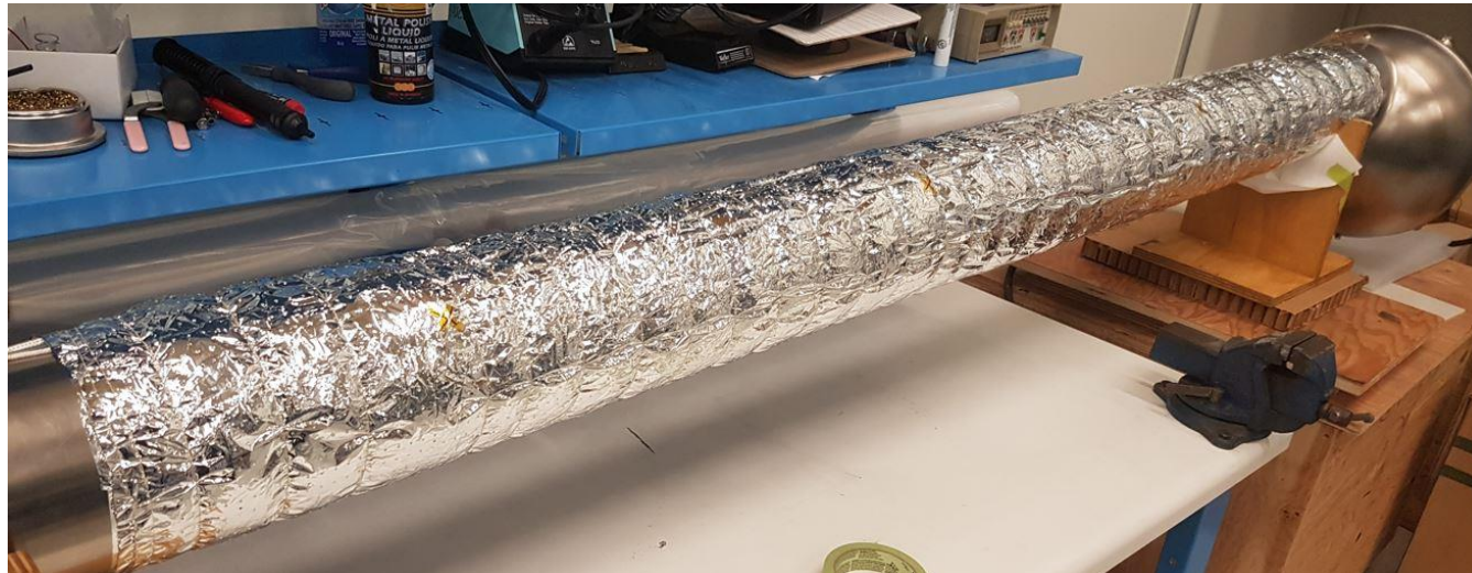
“Wall 1” in kapton super-insulation, all sensors installed
